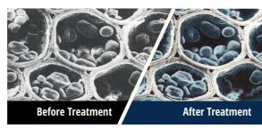
dassoCTECH is crystalized the fibers with CeramiX<sup>®</sup> particles, impregnated it with phenolic resin ( the same resin found in bowling balls ), then compressed to form Fused Bamboo. Because Fused Bamboo is now fully impregnated with CeramiX<sup>®</sup> particles that crystalizes the nutrients from attracting bacteria, fungus, molds or insects, the fibers does not rot under exposed environments.
